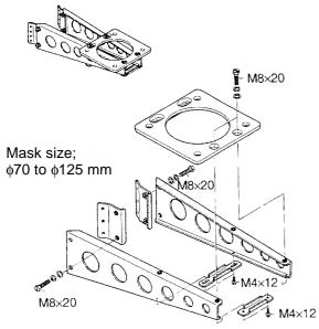
Type: OP03-92 Code no.: 008-445-070 Figure 5-3 Assembling the sailboat mast mounting bracket (option)
